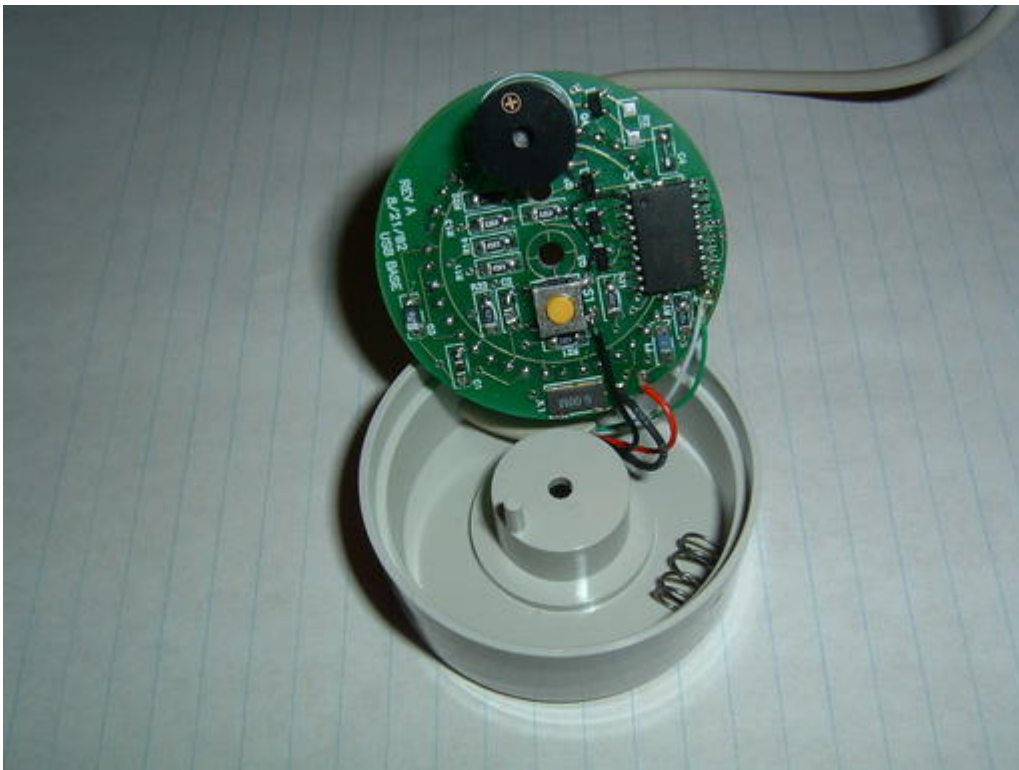
Figure 2. The three LEDs are connected to the first three pins of the controller chip.
