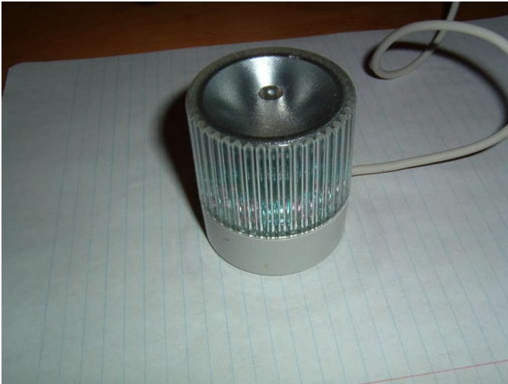
Figure 1. Delcom's USB Visual Signal Indicator is a simple first USB programming project.
